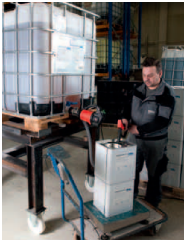
Fast container filling from the IBC outlet.
