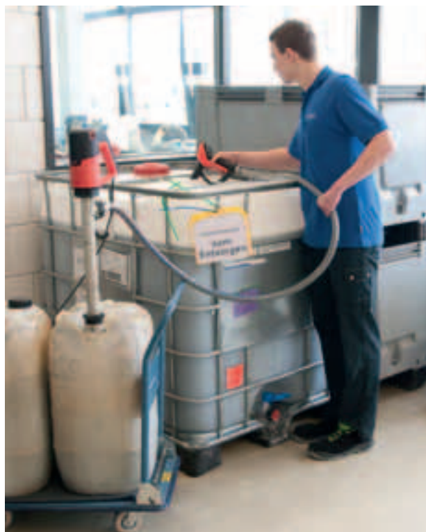
Disposal of mixed old chemicals (F 424 PP).
