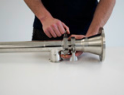
Open clamp on pump tube
