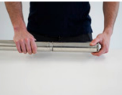
Unscrew stator housing
